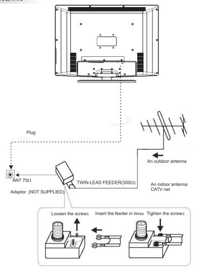
Note: Aerial connections: IEC(female). Input impendance:  $75\,\Omega$  unbalanced.
